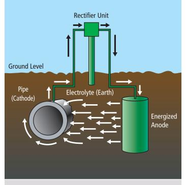
The system is designed, built and maintained to achieve the required electrical current flow in order to protect the steel pipeline from corrosion.
